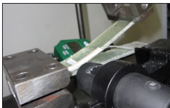
Fig. 2 MMF tests in the deformed configuration
