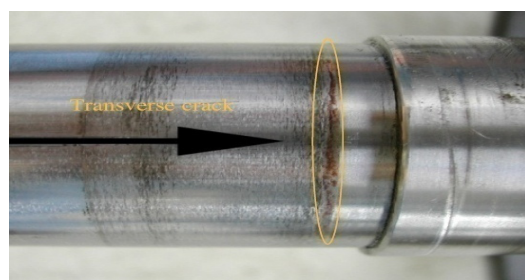
Fig. 1 A transverse crack [4]
