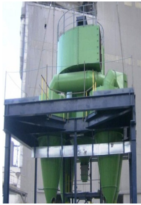
Fig. 1 A general view of the studied dynamic separator
